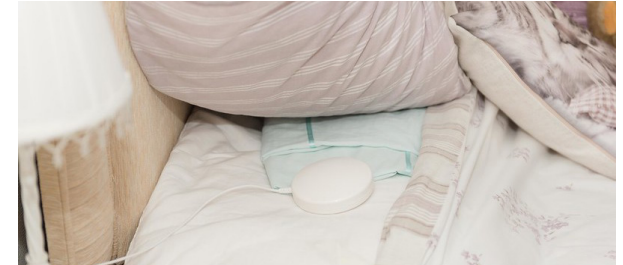
Photo: vibration device linked to smoke alarm
